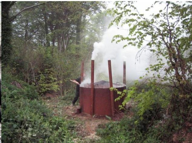
**Capturing Energy** – Today, biochar is produced using pyrolysis, that is, biomass is super-heated in the absence of oxygen at high temperatures (350-700°C) in specially designed furnaces. The most sustainable feedstocks are what's now considered waste: excess manure, wood debris, construction waste, slash from forest thinning, food processing waste, residue from methane digesters or urban tree trimmings. Most of this would be left to rot, be open-burned or dumped in a land fill.
