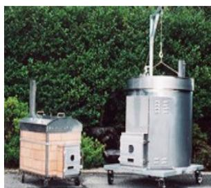
Japan, China and Australia innovated producing biochar in small pyrolysis ovens like those on the left. Great for residential use, these units dispose of waste, generate heat and power and produce biochar for the family garden. Stoves bigger than these can be converted to mobile units and taken to the biomass source saving on transportation costs when large amounts of biomass are available periodically but not regularly in a specific location.
